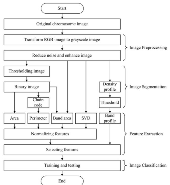
Figure 2. Image analysis block diagram.
